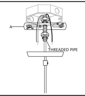
10. Slightly loosen ground screw on mounting bracket (A). Do not completely remove ground screw. Wrap house ground wire (copper) around ground screw, leaving enough ground wire to attach to fixture ground wire. Twist end of fixture ground wire and end of house ground wire (copper) together. Twist wire connector (C) onto ends of wires. Completely tighten wire connector (C). Reference chart below for correct wire connections.
