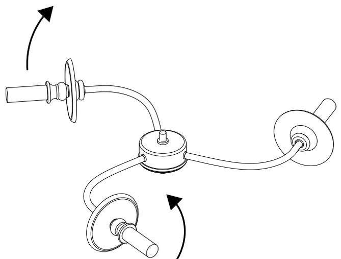
6. Pass fixture wires from top of fixture body (O) up through bottom of center stem (M). Pull fixture wires out of top of center stem (M). Carefully pull fixture wires taut.
