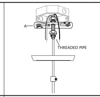
10. Slightly loosen ground screw on mounting bracket (A). Do not completely remove ground screw. Wrap house ground wire (copper) around ground screw, leaving enough ground wire to attach to fixture ground wire. Twist end of fixture ground wire and end of house ground wire (copper) together. Twist wire nut (C) onto ends of wires. Completely tighten wire nut (C). Reference chart below for correct wire connections.
